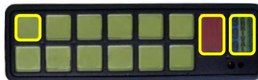
Keypad button press to enter/exit programming mode
